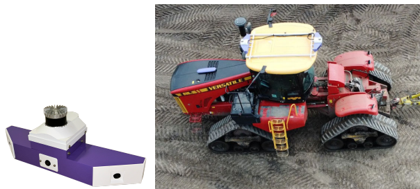
Fig. 1. An image of an example EYEBOS (left) with its 3 cameras and LiDAR sensor that can be mounted on a tractor. The right image shows a tractor with two EYEBOSs on its roof and a GNSS on its hood.
